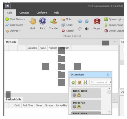
Docking hints are semi-transparent square elements that allow you to dock a panel to a form's edges, or to an existing container as a tab, or between other docking elements. These hints are displayed separately or grouped in a docking guide (e.g., in the ESI Communicator window's central area). Finally, a docking zone is a semi-transparent preview of exactly where your panel will be docked. This zone is displayed when you drag a panel into a docking hint, but before you drop it.
