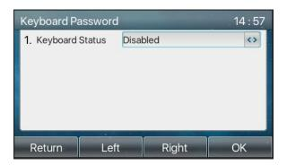
Once keyboard lock is set, long press # to lock the phone. A lock icon will appear in the top right corner of the screen. Phone will prompt "Enter Password" when any key is pressed.
