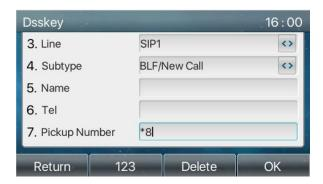
WEB interface: Log in the phone webpage, enter the [Function Key] page, select a DSSkey, set the key type as Memory Key, the subtype as BLF/NEW CALL, and set the corresponding SIP line and pick up codes. Click Apply to save.
