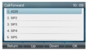
Select the call forward type by pressing the up/down navigation keys and press [OK].
