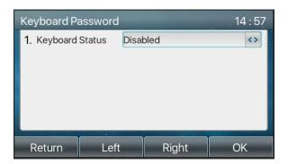
• Once keyboard lock is set, long press # at the home screen to lock the phone. A lock icon will appear in the top right corner of the screen. Phone will prompt "Enter Password" when any key is pressed.
