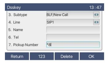
WEB interface: Log in the phone webpage, enter the [Function Key] page, select a DSSkey, set the key type as Memory Key, the subtype as BLF/NEW CALL, and set the corresponding SIP line and pick up codes.
