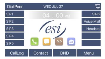
The image above shows the default standby screen, which is the user interface most of the time.
