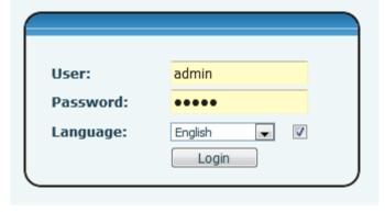
User must correctly enter the user name and password to log in to the web page. The default user name and password are "admin". For specific details on the web interface, refer to **Web Configurations** section.
