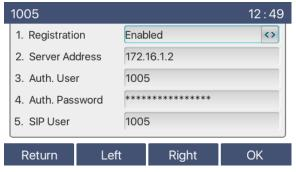
WEB interface: After logging into the phone page, enter [Line] >> [SIP] and select the line to configure from the drop down list. Enter SIP register information and click Apply to complete registration as shown below:
