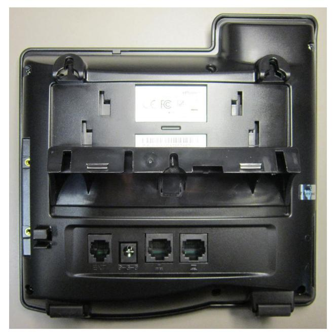
Use the template on the last page to mark and drill the mounting location. Use three wall anchors and three self-tapping screws to mount the phone to drywall. Slide the phone onto the wall making sure the three slots shown below engage the screws.
