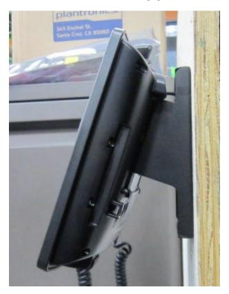
Make sure wall mount bracket locking tabs engage the ridge on the back of the phone.
