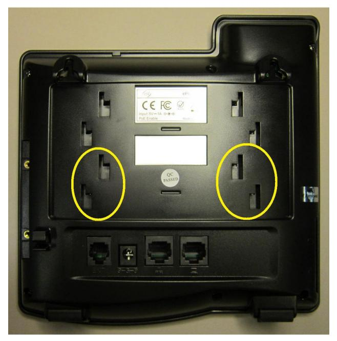
Slide the stand into the slots on the back of the phone as shown below.
