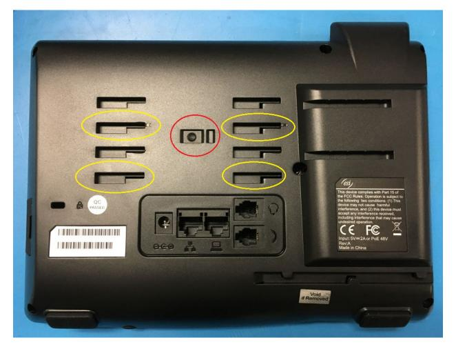
Slide phone onto bracket making sure tabs on the bracket engage the slots on the phone, and making sure that the locking tab fully engages the locking indentation, as shown below.
