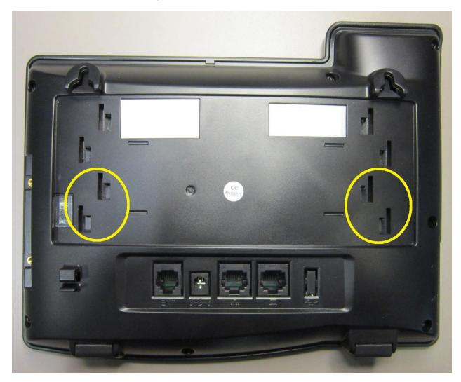
Locate the slots on the back of the phone onto which the stand will be mounted.
