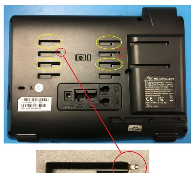
Locate the slots on back of phone (circled yellow). Also take note of the two indentations in the plastic (circled red), which will become apparent in the next step.
