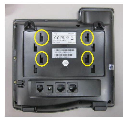
Install phone onto bracket. Make sure tabs on the bracket engage the slots on the phone.
