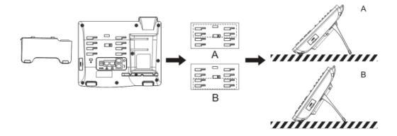
Orient handset hook to desired orientation as shown below.
